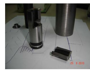
Fatal failure of a punch
