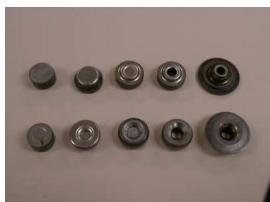
Punch failure during production of a valve spring retainer
