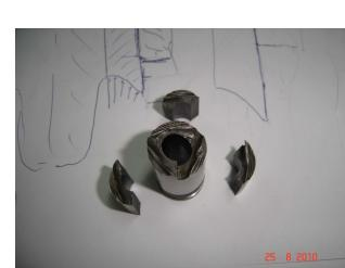
Fatal failure of a punch
