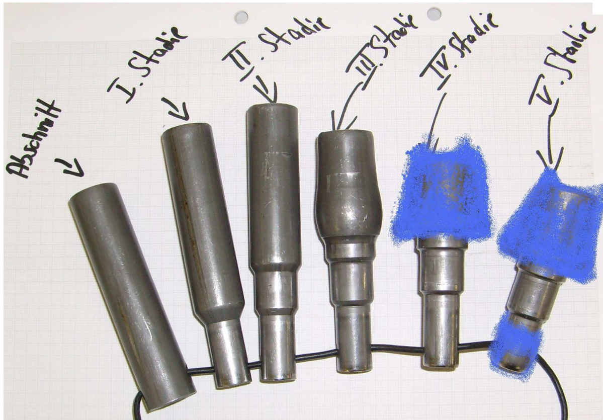
The five station cold forging process
