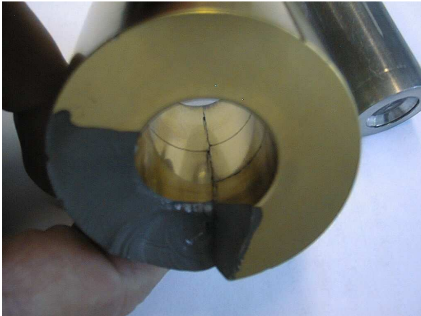
Figure 2: Die failing due to positive tangential stress
