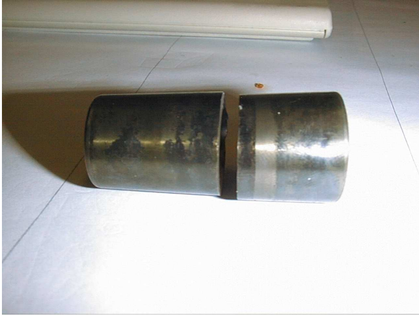
Figure 1: Die failing due to positive axial stress
