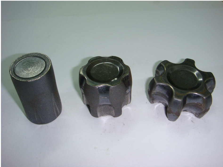
Figure 1: Operation one of forming an inner race (during process development)
