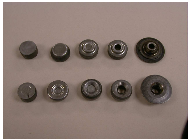
Figure 1: Progression to form the retainer
