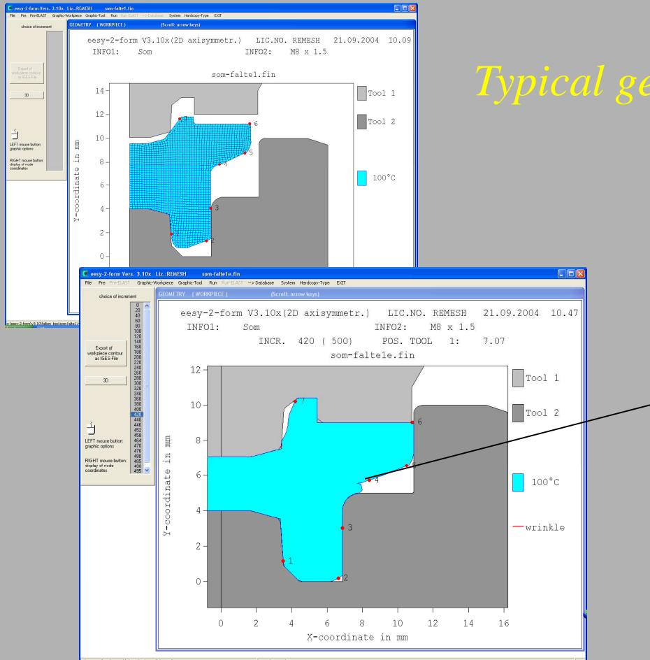
*Typical geom. failures in Process Design*
