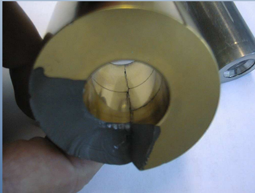
tool failure (die)
