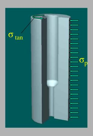
$\sigma_{tan}$ : critical for axial crack
