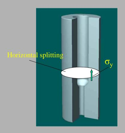
$\sigma_{y}$ : critical for horizontal crack
