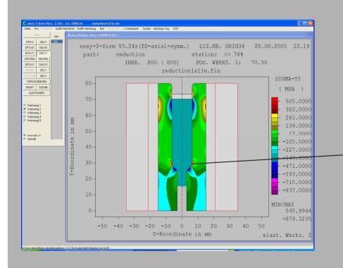
Avoiding of failures (elastic analysis of the insert with FEM)
