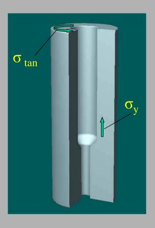
$\sigma_{tan}$ : critical for axial crack
