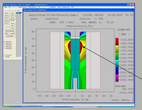
Design of a cold forming process
