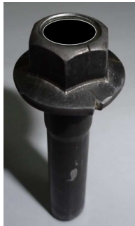
Crack in a screw (material failure)
