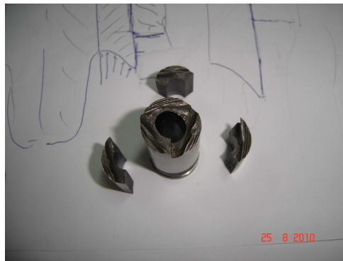
Fatal failure of a punch
