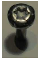
Cracks in a screw made from aluminum
