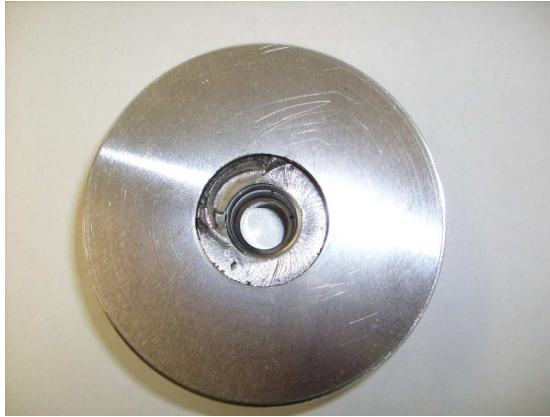
Premature tool failure in station 4: old layout
